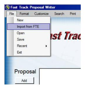
The software will search for the FTEC.mdb (or FTEC) database from Fast Track Estimating, which is the database that stores all created estimates. (It is best if the Fast Track Estimating software is closed when using this function.) The Fast Track Estimating Software should be installed in the C:\CPR\FTE directory. Make sure the date on the FTEC database (or FTEC) matches the last date changes were made to any estimate.
